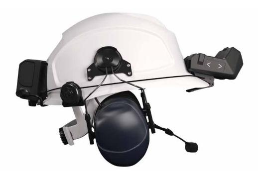
Kiber 3 Kit empowers field workforce with a wearable hardware for remote assistance based on AR technology: a head-mounted device with a unique binocular visor, an HD video camera, a high performances set of headphones/microphone and a 4GB local storage to store documents locally.
