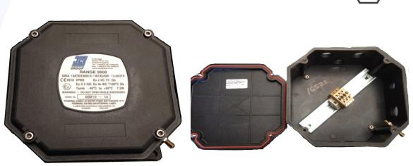
The JCE Group RANGE 9500 is an Explosion Protected/Weatherproof/Junction Box which is Sira certified under directive 94/9/EC (ATEX) for Group II, Category 2, G and D. The enclosure has been certified to give a large measure of flexibility based on Power Dissipation and is suitable for Zone 1, 2 (Gases) Zone 21 and 22 (Dusts).
