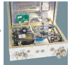
Interior view and typical bulkhead arrangement
